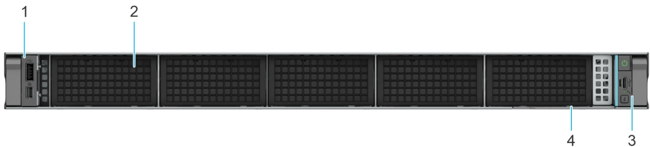
Figure 7. Front view of no backplane configuration system
