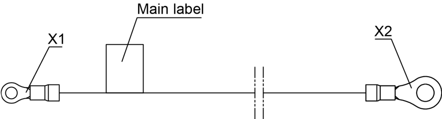
Figure 9-2 Structure of a ground cable
